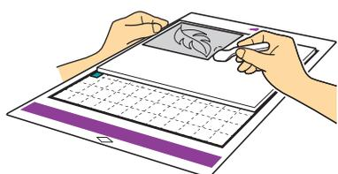
**10** (With metal sheets) Remove the metal sheet (with the protective sheets attached) from the embossing mat, and then peel both of the protective sheets from the metal sheet by using the tabs.
