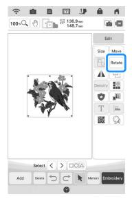
Select the key indicating the desired direction and angle for rotating the pattern. (Example: Totates 90 degrees clockwise.)
