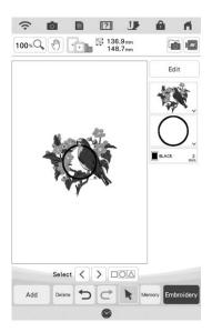
Press to edit the frame pattern to fit the size of the appliqué pattern.
