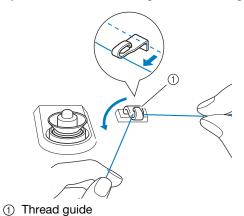
Pass the thread around the pretension disk making sure that the thread is under the pretension disk.
