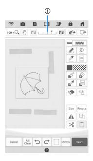
\* After the scanned image is converted to stitching, it appears as a background in the pattern drawing screen. Use gauge ① to adjust the transparency of the background. Each press of lightens the background, making the line pattern darker. Each press of darkens the background, making the line pattern lighter.
