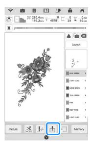
**7** Touch to set the starting point to the center of the pattern.
