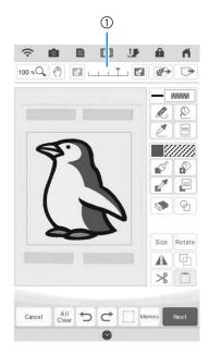
\* After the scanned image is converted to stitching, it appears as a background in the pattern drawing screen. Use gauge ① to adjust the transparency of the background. Each press of lightens the background, making the illustration pattern darker. Each press of darkens the background, making the illustration pattern lighter.
