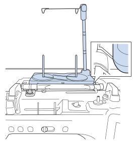
Place the spool of thread on the spool pin so that the thread feeds off the spool clockwise. Firmly insert the spool cap onto the spool pin.
