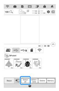
→ The thumbnails of selected patterns appear in blue. To deselect the pattern, either press the thumbnail again or press Select none.
