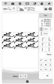
When changing the direction in which the pattern will be repeated, all of the patterns in the red frame will automatically be grouped as one repeating unit. Refer to the following section on how to repeat one element of a repeated pattern.
