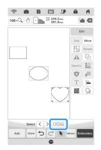
Press Edit , , and then press the key for the desired alignment.
