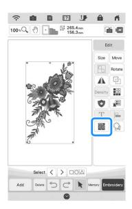
→ Stippling is automatically applied around the selected pattern.
