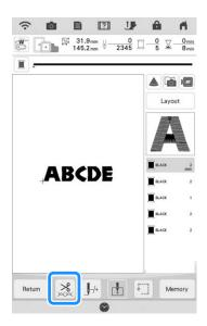
6 Press ► to turn off the thread cutting function and then press .
