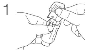
1 Press the button at the center of the pen holder to unhook the lid and open it.
