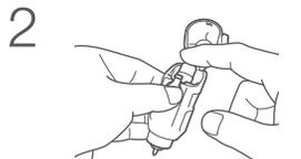
2 Remove the cap from the pen, insert the pen into the pen holder with the point down, and then close the pen holder's lid.
