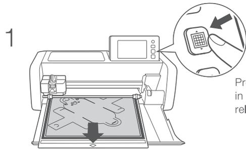
1 Press the "Feed" button in the operation panel to release the mat.
