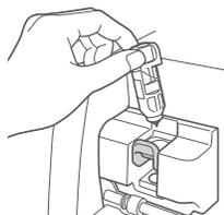
Raise the holder lock lever, remove the pen holder. Properly store the pen by removing the pen from the pen holder and attach the pen's cap.
