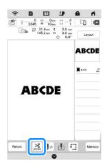
Press to turn off the thread cutting function and then press ok.
