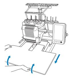
After the pins on each side reach the notches in the guide plates, raise the wide table to lift the pins up through the notches.
