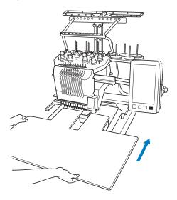
While looking below the wide table, lightly lift it up, and then lower it so that the screw fits into the notch at the front of the guide plate.
