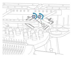
Turn the screw counterclockwise three or four times to loosen it. Grab the grips on the thread guide assembly support and push toward the middle.
