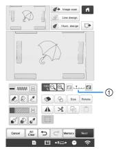
\* After the scanned image is converted to stitching, it appears as a background in the pattern drawing screen. Use gauge ① to adjust the transparency of the background. Each touch of I lightens the background, making the line pattern darker. Each touch of darkens the background, making the line pattern lighter.
