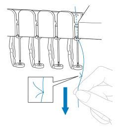
Continue pulling the thread until the knot is below the needle. Cut the knot.
