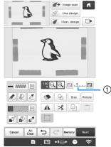
\* After the scanned image is converted to stitching, it appears as a background in the pattern drawing screen. Use gauge ① to adjust the transparency of the background. Each touch of I lightens the background, making the illustration pattern darker. Each touch of darkens the background, making the illustration pattern lighter.
