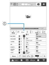
① Time until the machine stops
