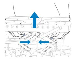
After the thread guide assembly support is extended and the thread guide assembly is raised to its highest position, tighten the two thumb screws to secure the thread guide assembly in place.
