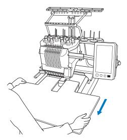
Tighten the thumb screws on the wide table.
