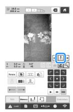
Touch the positioning keys to move the embroidery frame until the thread mark on the fabric is aligned on the needle drop point in the camera view window.
