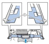
① Make sure that the pins on the left and right arms of the embroidery frame holder fit into the positioning slot and hole on the embroidery frame.
