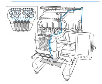
On the spool pin, place a spool with the thread color specified for the corresponding needle bar.
