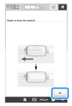
If you want to rehoop the fabric while the camera image is being displayed, touch . After the on-screen instructions appear, rehoop the fabric.
