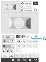
\* After the scanned image is converted to stitching, it appears as a background in the pattern drawing screen. Use gauge ① to adjust the transparency of the background. Each touch of I lightens the background, making the line pattern darker. Each touch of darkens the background, making the line pattern lighter.
