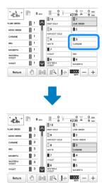
→ The thread color sequence display and pattern for the thread color of the selected needle bar appear.
