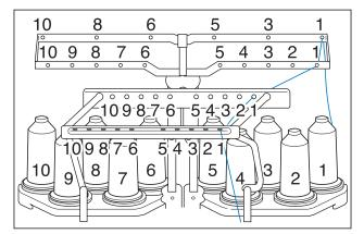
Pass the thread of a specified color through the holes on the thread guide, making sure that you have the thread color matched to the coordinating needle bar. Pass the thread from spool pins 1, 3, 5, 6, 8 and 10 through the holes in both thread guides A and B. Pass the thread from spool pins 2, 4, 7 and 9 through the hole in thread guide B only.
