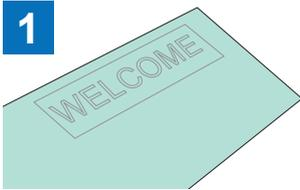
1 Half-cut the desired pattern with the cutting machine.
