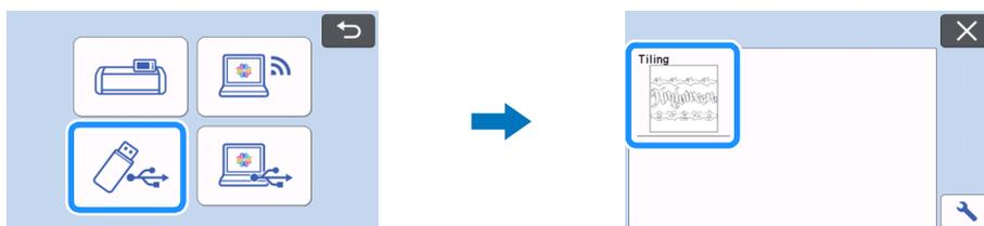
**9 Select the first pattern of the tiled data to be cut, and then touch the "OK" key.**
