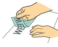
3 Attach the application sheet <sup>\*1</sup> to the area of the backing where the pattern remains. (<sup>\*2</sup>)
