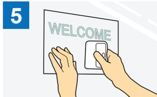
5 After wiping the target surface clean, attach the adhesive craft vinyl cutouts with the application sheet. (<sup>\*2</sup>)
