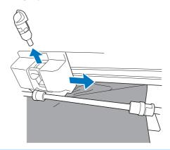
6 Return the feeder release lever (on the right side of the machine) to its original position.
