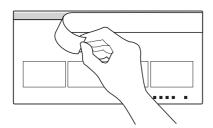
3 Attach the material from above by aligning it straight along the attachment position line (black line) on the leader sheet. At this time, align the leader sheet and the left side edge of the material and stick them together.
