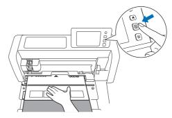
When the material is fed into position, preparation of the roll feeder is completed. At this time, make sure that the left and right feed rollers completely pass over the leader sheet.
