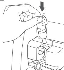
Grasp the grip, and then firmly insert the holder into the carriage.
