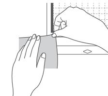
Normally, before attaching material to the mat, test attaching the material to an edge of the adhesive side of the mat in order to check that the appropriate mat was selected. However, for this project, test attaching with the enclosed paper is unnecessary.
