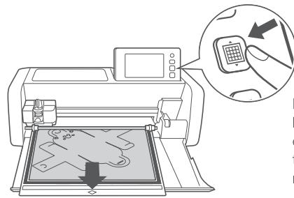
Press the "Feed" button in the operation panel to release the mat.
