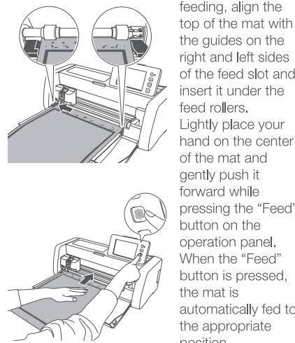
For smooth feeding, align the top of the mat with the guides on the right and left sides of the feed slot and insert it under the feed rollers. Lightly place your hand on the center of the mat and gently push it forward while pressing the "Feed" button on the operation panel. When the "Feed" button is pressed, the mat is automatically fed to the appropriate position.
