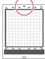
Make sure that the arrow is facing the machine feeder (top side up).
