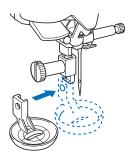
6 Tighten the screw with the included screwdriver (large).
