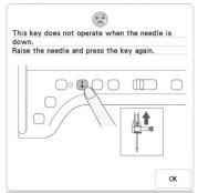
This message is displayed when a key on the LCD display is touched while the needle is in the down position.
