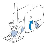
When the feed position lever is down, the black roller belt on the dual feed is engaged.
