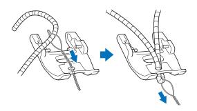
Attach the couching dual feed foot shown below to the dual feed foot.
