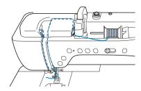
Pass the thread through the needle bar thread guide on the needle bar, then thread the needle on the left side manually.
