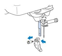
Set the adapter on the presser foot bar, aligning the flat side of the adapter opening with the flat side of the presser foot bar. Push it up as far as possible, and then tighten the screw securely with the screwdriver.
