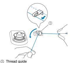
Pass the thread around the pretension disk making sure that the thread is under the pretension disk.
