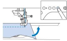
The pivot setting is useful when changing the sewing direction. When the machine is stopped at the corner of the fabric, the machine stops with the needle in the fabric and the presser foot is automatically raised so the fabric can easily be rotated ("Pivoting" on page 89).
