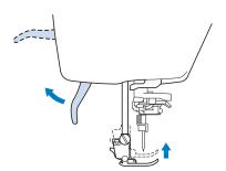
Press the black button on the presser foot holder and remove the presser foot.
