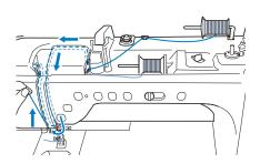
Continue threading; however, do not pass the thread in the needle bar thread guide "6" on the needle bar. Thread the needle on the right side.
