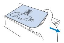
6 Insert the tabs on the straight stitch needle plate into the notches in the machine.
