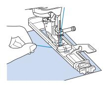
→ Once sewing is completed, the machine automatically sews reinforcement stitches, and then stops.
