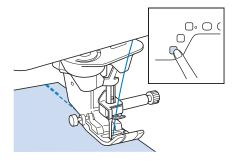
Press the "Thread Cutter" button to trim the upper and lower threads.
