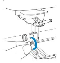
6 Set the operation lever of the walking foot so that the needle clamp screw is set in the fork. Position the shank of the walking foot on the presser foot bar.
