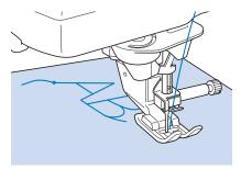
After sewing is finished, use a seam ripper to trim any excess thread (jump stitches).
