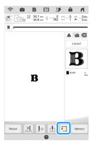
Press — to set the starting point to the center of the pattern.
