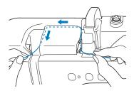
Guide the thread down, up, then down through the groove, as shown in the illustration.
