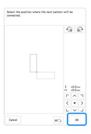
→ Message appears on screen and carriage will move after pressing ox.
