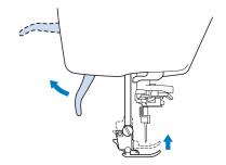
Press the black button on the presser foot holder and remove the presser foot.
