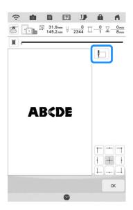
→ The needle is positioned in the lower-left corner of the pattern. The carriage moves so that the needle is positioned correctly.
