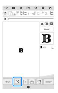
Press — to loosen the upper thread tension. (The tension number will decrease.)
