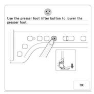
This message is displayed when a button, such as the "Start/Stop" button, is pushed while the presser foot is raised.
