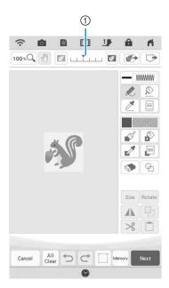
\* After tracing elements of the imported image and assigning stitch patterns to the lines and regions, the image appears as a background in the pattern drawing screen. Use gauge ① to adjust the transparency of the background. Each press of lightens the background, making the line pattern darker. Each press of darkens the background, making the line pattern lighter.
