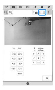
Press the positioning keys to move the embroidery frame until the thread mark on the fabric is aligned on the starting point in the camera view window.
