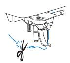
If the thread is left at the beginning of the stitching, it may be embroidered over as you continue embroidering the pattern, making it very difficult to remove the excess thread after the pattern is finished. Trim the thread at the beginning.
