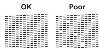
Follow the LCD instructions to check the quality of the four color blocks on the sheet, and then start the cleaning procedure.
