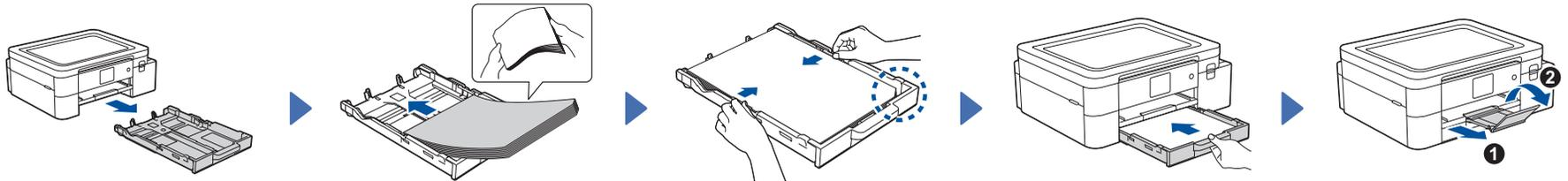
Pull the paper tray completely out of the machine.
