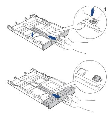
4. Gently press and slide the paper width guides (1) and the paper length guide (2) to fit the paper size.
