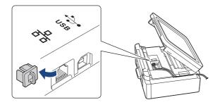
Carefully guide the cable through the cable channel and out the back of the machine.
