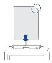
5. Using both hands, push **one sheet of paper** into the manual feed slot until the front edge touches the paper feed rollers. Release the paper when you feel the machine pull it. The LCD displays [Manual Feed Slot ready]. Follow the instructions displayed on the LCD.
