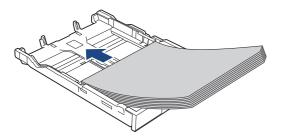
Make sure the paper is flat in the tray and the paper length guide (1) touches the edges of the paper.
