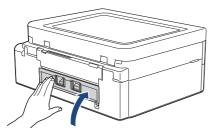
5. Put the paper support firmly back in the machine. Make sure you fit the paper support into the channels.
