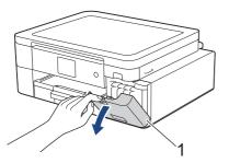
2. Press the lock release lever to release the ink cartridge colour indicated on the LCD and remove the ink cartridge from the machine, as shown in the illustration.
