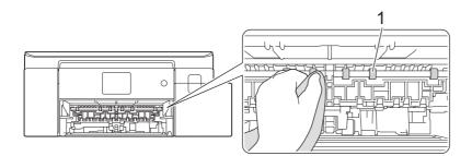
6. Put the paper support firmly back in the machine. Make sure you fit the paper support into the channels.
