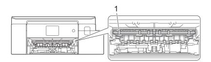
b. Squeeze both levers (1), and then open the Jam Clear Cover at the back of the machine.
