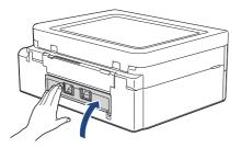
7. Put the paper support firmly back in the machine. Make sure you fit the paper support into the channels.
