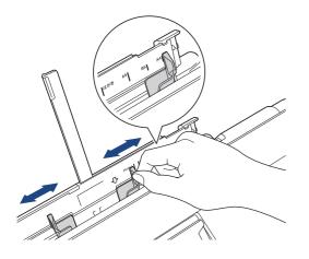
Load only one sheet of paper in the manual feed slot with the printing surface face up.
