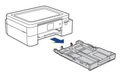
3. Press the square paper tray expansion button (1) and slide out the paper tray until the square paper tray expansion button locks into the square LGL hole.
