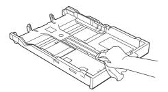
6. Wipe the outside of the paper support with a dry, lint-free cloth to remove dust.
