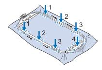
Gently smooth out the fabric. With the lever at the bottom loosened, slightly tighten the frame adjustment screw, and then pull the edges of the fabric to remove any slack.
