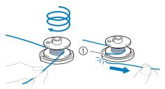
Guide slit in bobbin winder seat (with built-in cutter)
