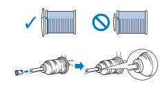
4 With your right hand, hold the thread near the thread spool. With your left hand, hold the end of the thread, and use both hands to pass the thread through the thread guide.
