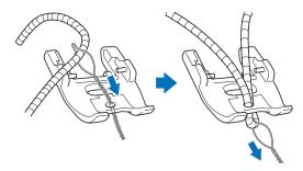
7 Attach the couching dual feed foot shown below to the compact dual feed.
