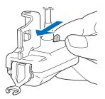
Correctly orient the presser foot, insert it horizontally into the presser foot slot, and then push it in as far as it will go.
