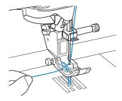
Pull up the bobbin thread, pass it under the presser foot and pull it about 10 cm (approx. 4 inches) toward the back of the machine, making it even with the upper thread.
