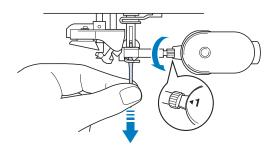
With the flat side of the needle facing the back, insert the new needle until it touches the needle stopper. Use a screwdriver to securely tighten the needle clamp screw.
