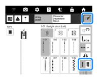
→ Twin needle mode is set. Only stitch patterns that allow twin needle sewing can be selected.
