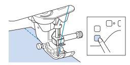
9 Press (Thread cutter button) to trim the upper and bobbin threads.
