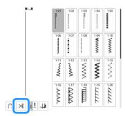
→ The keys will display as , and the machine is set for automatic thread cutting function and automatic reverse/reinforcement stitching.
