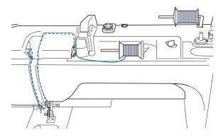
Pass the thread through the needle bar thread guide, then thread the needle on the left side manually.
