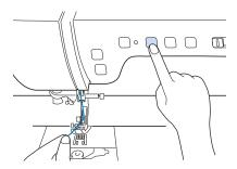
5 Press (1) (Needle position button) to raise the needle.
