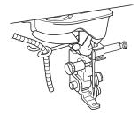
13 Thread the yarn through embroidery couching foot "Y". Pass the yarn through the loop in the yarn threader, and then pass the threader from top to bottom through the hole in embroidery couching foot "Y". Pull the yarn to the front of the machine.
