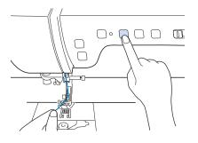
Press (1) (Needle position button) to raise the needle.
