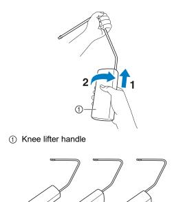
2 Align the tabs on the knee lifter with the notches in the knee lifter slot on the front of the machine. Insert the knee lifter bar as far as possible.
