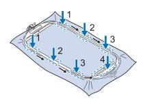
5 Gently smooth out the fabric. With the lever at the bottom loosened, slightly tighten the frame adjustment screw, and then pull the edges of the fabric to remove any slack.
