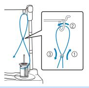
4 Pass the thread through the machine's thread guide from the right to the left.
