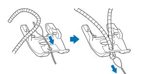
7 Attach the couching dual feed foot shown below to the compact dual feed.
