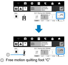
4 Remove the presser foot holder. (page 48) 5 Attach free motion quilting foot "C" as shown the illustration and tighten the presser foot holder screw.
