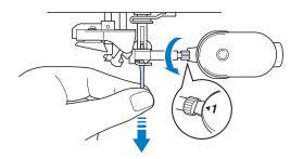
5 With the flat side of the needle facing the back, insert the new needle until it touches the needle stopper. Use a screwdriver to securely tighten the needle clamp screw.
