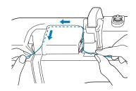
8 Guide the thread down, up, then down through the groove, as shown in the illustration.
