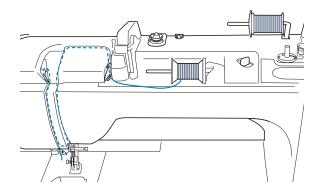
**3** Pass the thread through the needle bar thread guide, then thread the needle on the left side manually.
