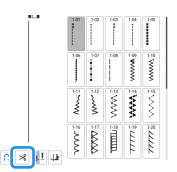
→ The keys will display as A >>>, and the machine is set for automatic thread cutting function and automatic reverse/reinforcement stitching.
