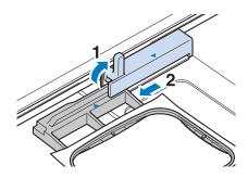
Insert a wound bobbin into the machine. (Refer to "Setting the Bobbin" on page 40.)
