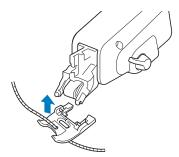
8 Pull out the yarn for about 10 cm (approx. 4 inches) to the back of the machine.
