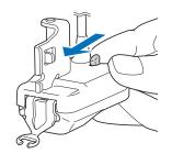
7 Correctly orient the presser foot, insert it horizontally into the presser foot slot, and then push it in as far as it will go.
