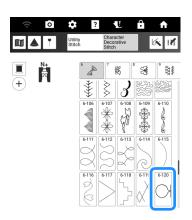
2 Attach advanced monogramming foot "N+" and sew the stitch pattern. Compare the finished stitch pattern to the illustration of the correct stitch pattern below. Touch , and then adjust the stitch pattern with the [Fine Adjust Verti.] or [Fine Adjust Horiz.] displays.
