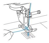
7 Pull up the bobbin thread, pass it under the presser foot and pull it about 10 cm (approx. 4 inches) toward the back of the machine, making it even with the upper thread.
