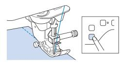
9 Press  $(\gg)$  (Thread cutter button) to trim the upper and bobbin threads.
