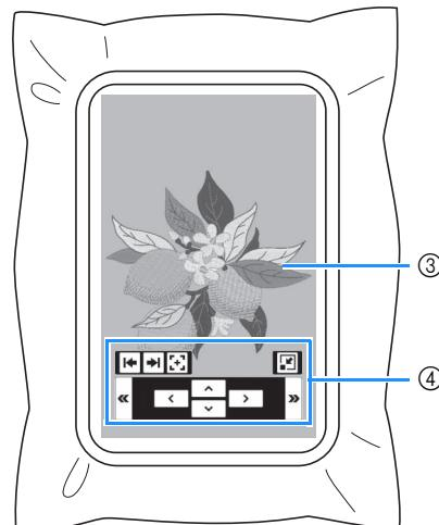
① Drag a blue line at one of the four corners to move the embroidery frame and change the location of the projection area on the fabric.
