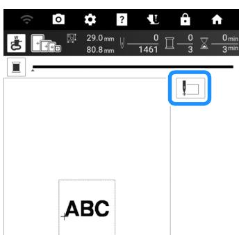
→ The needle is positioned in the lower-left corner of the pattern. The embroidery frame will move to the specified needle position.
