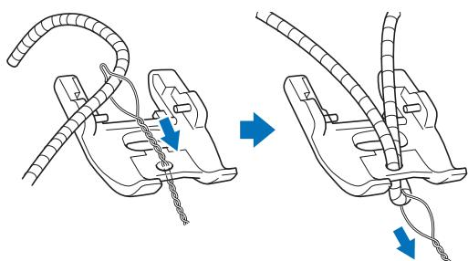
**7 Attach the couching dual feed foot shown below to the compact dual feed.**
