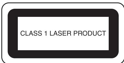
The invisible laser beam emitted by the laser unit installed in this stitch regulator is restricted to an output at a safe level. The stitch regulator contains 0.6-milliwatt, 840-860 nanometer wavelength, 1.5 mrad divergence angle, pulse duration 26  $\mu$ s, pulse frequency 10 kHz, laser module. However, eye damage may result from disassembling or altering this stitch regulator. Safety precautions have been designed to prevent any possible laser beam exposure to the operator.
