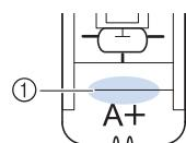
**4** Check the first needle drop point and lower the presser foot.
