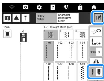
→ Twin needle mode is set. Only stitch patterns that allow twin needle sewing can be selected.
