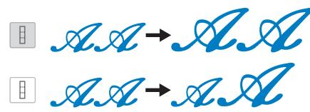
② When the maintain aspect ratio key appears as
