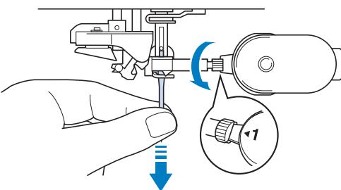
**5** With the flat side of the needle facing the back, insert the new needle until it touches the needle stopper. Use a screwdriver to securely tighten the needle clamp screw.
