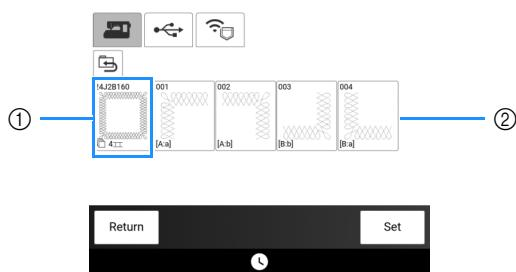
① To embroider using the built-in camera for aligning the embroidering position, touch the key showing the entire pattern.
