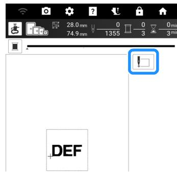
→ The carriage moves so that the needle is positioned in the lower-left corner of the pattern. You will need to match this point to the end of embroidering for the previous pattern.
