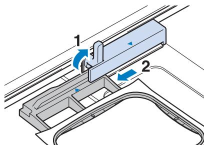
**6** Insert a wound bobbin into the machine. (Refer to "Setting the Bobbin" on page 40.)
