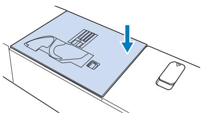
**4** If necessary, attach the flat bed attachment.
