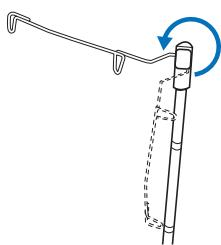
**4 Open the upper cover of the machine, and then place the spool stand on the upper cover as shown in the illustration.**
