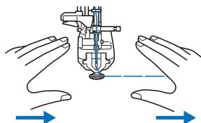
→ Stitches will be sewn at the set stitch length in response to the speed at which the fabric is moved.
