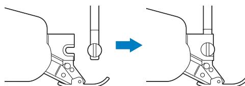
4 Hold the compact dual feed foot in place with your right hand, then using the included multi-purpose screwdriver, securely tighten the screw.
