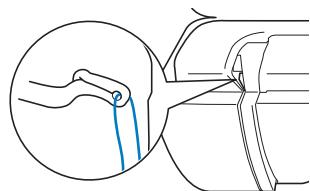
**9** Pass the thread through the needle bar thread guide (marked "6") by holding the thread with both hands and guiding it as shown in the illustration.
