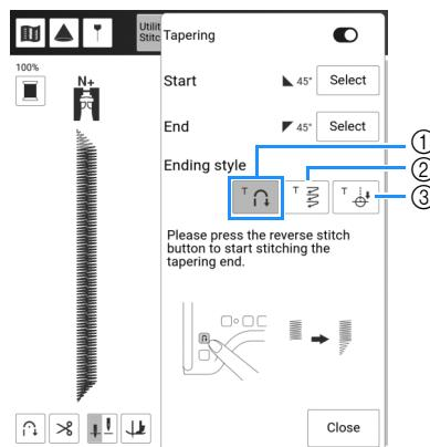
① Press (Reverse stitch button) for the angle at the end of sewing to start changing; the machine stops when sewing is finished.
