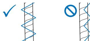
**3 Rotate the handwheel to set the needle in the sewing start position. Start sewing on the right side of the yarn.**
