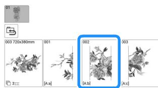
7 Rehoop the fabric. Adjust the position and angle for the next pattern so that the alignment stitching embroidered with the first pattern and the needle position for the next pattern are aligned. For this example, touch , select the upper-left needle position, and then touch [OK].
