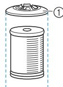
When using thread on a thin spool, place the included spool felt (①) on the spool pin, place the thread spool on the spool pin so that the center of the spool is aligned with the hole at the center of the spool felt, and then insert the spool cap onto the spool pin.
