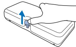
**2** Fully extend the telescopic thread guide shaft until the two internal stoppers snap into place.
