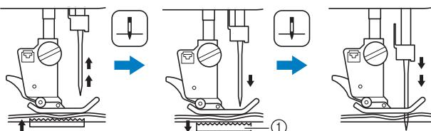
① The feed dogs are lowered. At this time, the fabric can be shifted to finely adjust the needle drop point.
