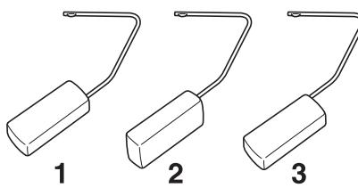
**2** Align the tabs on the knee lifter with the notches in the knee lifter slot on the front of the machine. Insert the knee lifter bar as far as possible.
