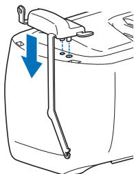
**11 Pass the yarn through the telescopic thread guide and the yarn guide (①) to (②).**
