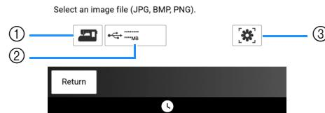
① The most recently scanned image is automatically stored in the machine's memory. Touch this key to import the scanned image.
