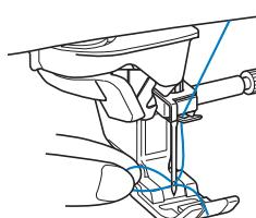
**15** Raise the presser foot and pull out about 10 cm (approx. 4 inches) of the thread, and then pass it under the presser foot toward the rear of the machine.
