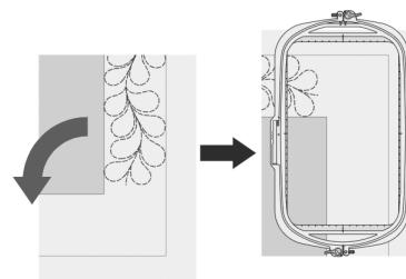
Use the move pattern keys to align the start point projected by the projector with the end point of the previous pattern, and then touch [OK].
