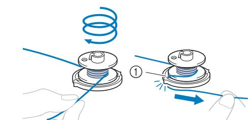
① Guide slit in bobbin winder seat (with built-in cutter)
