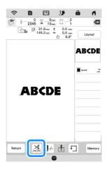
Touch ♣ to turn off the thread cutting function and then touch ok .
