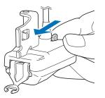
Correctly orient the presser foot, insert it horizontally into the presser foot slot, and then push it in as far as it will go.
