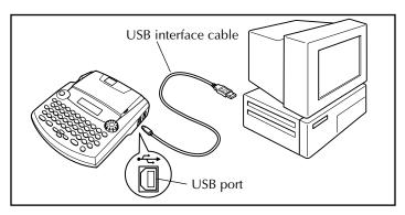
After the P-touch is connected to a computer using a USB cable, the P-touch enters Interface mode when data is sent from the computer.
