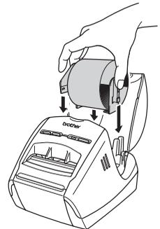
**3** Thread the end of the DK Roll into the slot until it aligns to the area shown right.
