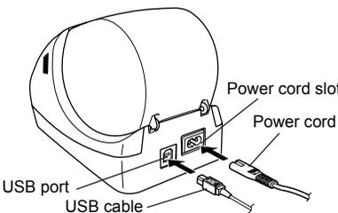
The diagram shows the back of the P-touch Editor machine. A power cord is plugged into a power cord slot. A USB cable is plugged into a USB port. A caution label is shown being removed from the USB port.
