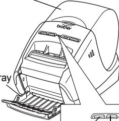
FEED button CUT button LED lamp ON/OFF button
