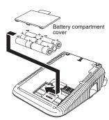
Attach the battery compartment cover by inserting the three hooks at the bottom into the slots on the machine, then pushing down firmly on the cover until it snaps into place.
