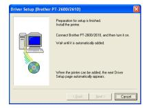
Connect the P-touch 2600/2610 to the computer using the enclosed USB interface cable as described on page 6, and then turn on the P-touch 2600/2610. The first Found New Hardware Wizard dialog box appears.
