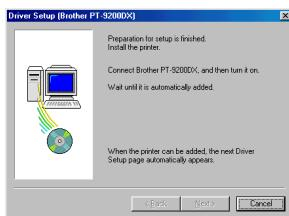
Connect the PT-9200DX to the computer using the enclosed USB interface cable as described on page 5, and then turn on the PT-9200DX. A dialogue box appears, showing that the printer driver has been installed.
