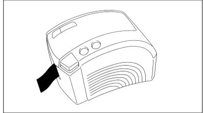
Using a cotton swab dipped in isopropyl (rubbing) alcohol, clean off the metal piece in the exit slot to the left of the cutter.
