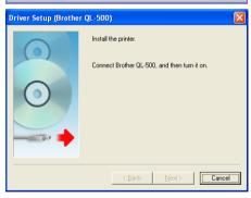
When the Driver Setup dialog box instructs you to connect the QL-500/ 550, plug the connector on the USB cable into the USB port on the back of the QL-500/550.
