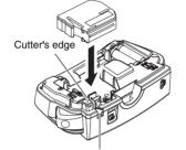
· Make sure that the end of the tape feeds under the tape guides. • Use only Brother M tapes with this machine.
