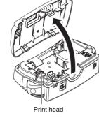
Insert four new AAA-size alkaline batteries (LR03), making sure that their poles point in the correct directions. Always replace all four batteries at the same time using brand
