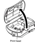
Insert four new AAA-size alkaline batteries (LR03), making sure that their poles point in the correct directions. Always replace all four batteries at the same time using brand
