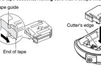
· Make sure that the end of the tape feeds under the tape guides. · Use only Brother M tapes with this machine.
