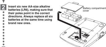
Attach the battery compartment cover by inserting the three hooks at the bottom into the slots on the machine, then pushing down firmly on the cover until it snaps into place.
