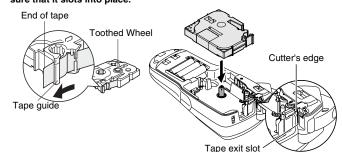
Make sure that the end of the tape feeds under the tape guides. • If the ink ribbon is loose, use your finger to wind the toothed wheel in the direction of the arrow on the cassette.
