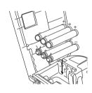
Insert six new AAA alkaline batteries (LR03), making sure that their poles point in the correct directions. Always replace all six batteries at the same time using brand new
