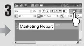
Enter the desired text and click the **Print** button. The tape will advance and place cut marks where the margin should be manually cut to accommodate small margins.
