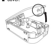
Verify that the P-touch labeller is turned off. Open the cassette cover as shown by the arrow in the above illustration while pressing the part marked "<<".
