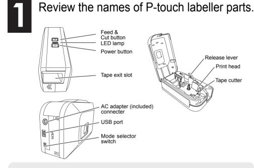
The PT-2430PC has 2 mode selector settings - "EL" and "E". The mode selector switch is pre-set at the factory to the EL mode, for use with P-touch Editor Lite. For E mode, you will need to install P-touch Editor 5.0, a more advanced labeling software, and the required drivers from the enclosed CD. For details on how to install P-touch Editor 5.0, see "Starting P-touch Editor 5.0" below.
