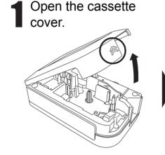
Verify that the P-touch labeller is turned off. Open the cassette cover as shown by the arrow in the above illustration while pressing the "<<" section of the tape cover.
