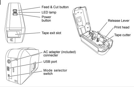
The PT-2430PC has 2 mode selector settings - "EL" and "E". The mode selector switch is pre-set at the factory to the EL mode, for use with P-touch Editor Lite. For E mode, you will need to install P-touch Editor 5.0, a more advanced labeling software, and the required drivers from the enclosed CD. For details on how to install the P-touch Editor 5.0, see "Starting P-touch Editor 5.0" below
