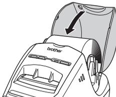
Close the DK Roll Compartment cover and press the ON/OFF button to turn the machine ON. Press the FEED and CUT buttons (if necessary) to properly align paper.
