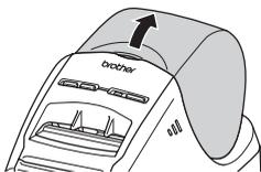
Press and hold the ON/OFF button to turn off the machine. Firmly hold the front of the machine and lift open the DK Roll compartment cover.
