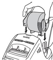
Put the new spool into the spool guides of the DK Roll compartment.
