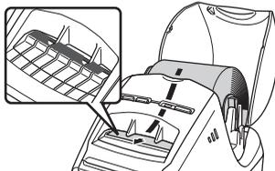
Thread the end of the DK Paper Roll all the way through the slot as shown in the illustration.
