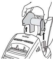
Remove the empty spool by lifting up and out of the machine.
