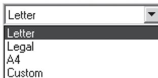
For standard paper sizes, this setting determines default margins and expected length for each printed page. For 'Custom' sizes, margins and length may be set using the commands 'Form Length', 'Bottom Margin', 'Left Margin' and 'Right Margin'.
