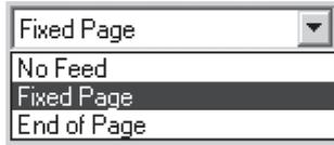
This setting affects what the printer will do in response to a Form Feed command from any source. Different modes are appropriate depending upon the type of paper being used.
