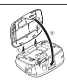
Insert the two hooks at the bottom of the cassette cover into the slots on the machine (1), and then close the cover securely until it snaps into place (2).
