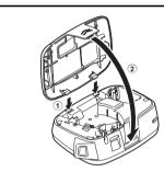
Insert the two hooks at the bottom of the cassette cover into the slots on the machine (1). and then close the cover securely until it snaps into place (2).
