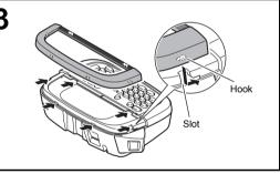
Insert the hooks on the front cover into the slots on the machine, and slide the cover back into place.
