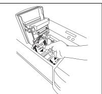
For a jam near the xenon lamp unit ("REMOVE LABEL 3" appears on the display):
