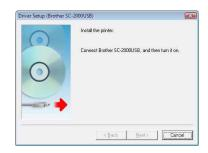
When this Driver Setup dialog box appears, connect a USB cable from your computer to the SC-2000USB. Then turn the SC-2000USB on.
