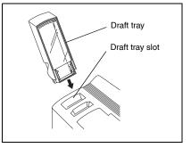
After installing the ink ribbon cassette and the draft tray loaded with draft sheets, you can use P-touch Editor software or Stampcreator Express software to create any layout containing graphics and text, and then engrave it into a stamp.
