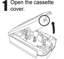
Verify that the P-touch labeller is turned off. Open the cassette cover as shown by the arrow in the above illustration while pressing the "<<" section of the tape cover.
