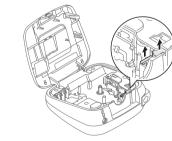
2. Install a new Cutter Unit. Push it in gently until it snaps into place.
