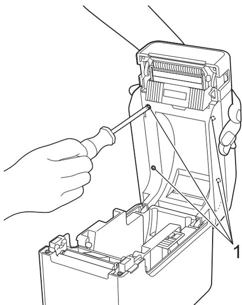
**!** Be careful not to allow the top cover to fall when the four screws are removed.
