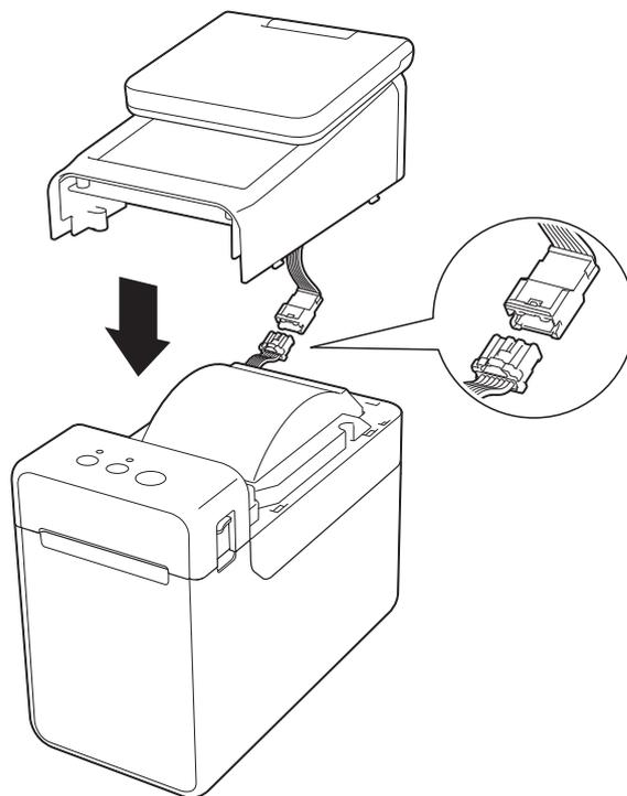
**!** Be careful that the connector cords are not trapped by the cover. In addition, if the cords are caught between the screw holes, the cords may be damaged when the screws are tightened.
