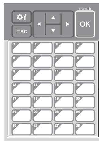
The data registered with each key in the one-touch panel is determined by the key number. If the one-touch panel will be used, the number must be specified before the data is transferred.
