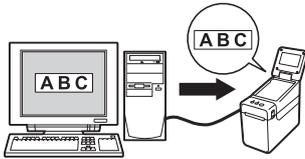
Use P-touch Transfer Manager to transfer the created label layout from the computer to the printer.
