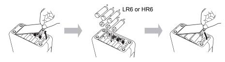
To remove the batteries, reverse the installation procedure.
