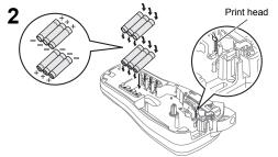
Insert six new AAA alkaline batteries (LR03) or fully charged Ni-MH batteries (HR03), making sure that their poles point in the correct directions. Users of alkaline batteries: Always replace all six batteries at the same time with brand new ones.
