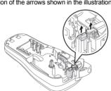
2. Install a new cutter unit. Push it in until it snaps into place.
