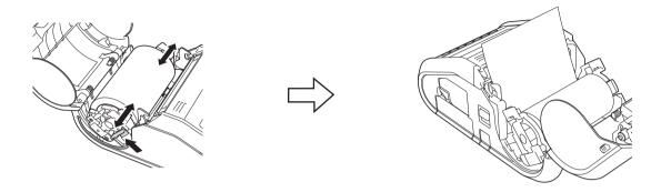
4 Close the RD Roll compartment by pressing down on the centre of the cover until it latches.
