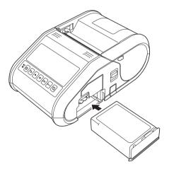
With the battery inserted and while pushing the battery lightly into the cavity, lower the battery latch until it clicks locking the battery in place.
