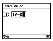
5 For the second serialised text, select [Type], [Format], [From], [To] and [Increased by] using the ↑ or ↓ key, set the values using the ← or → key, and then press the OK or Enter key.
