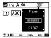
3 Select a frame using the ↑ or ↓ key, and then press the **OK** or **Enter** key. The selected frame is inserted.
