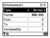
3 For the first serialised text, select [Type], [Format], [From], [To] and [Increased by] using the ↑ or ↓ key, set the values using the ← or → key, and then press the **OK** or **Enter** key.
