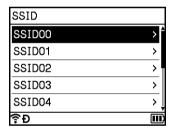
7 Select the SSID using the ↑ or ↓ key, or select [Other...] and enter the SSID (from 1 to 32 characters), and then press the **OK** or **Enter** key.
