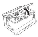
2 Pull the tube release lever up.
