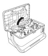
3 Pass the tube as shown in the illustration so that the end of the tube reaches the " ← c " mark on the P-touch, and then push the tube release lever down.
