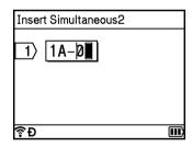
For the second serialised text, select [Type], [Format], [From], and [Increased by] using the ↑ or ↓ key, set the values using the ← or → key, and then press the OK or Enter key.
