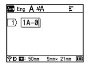
2 Position the cursor where you want to insert the first serialised text (to the right of "0"), and then press the Shift and Serialize keys. Select [Simultaneous] using the ↑ or ↓ key, and then press the OK or Enter key.
