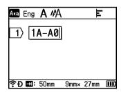
2 Position the cursor where you want to insert serialised text, and then press the Serialize key.
