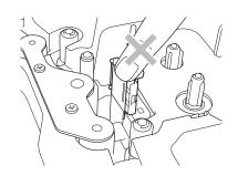
DO NOT touch any metal parts near the print head. The print head becomes very hot during and immediately after use. DO NOT touch it directly with your hands.
