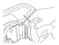
■ DO NOT touch the blade of the tube cutter unit.
