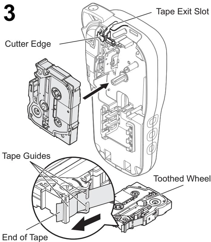
**Insert the Tape Cassette following the drawing marked inside the case. Gently press the Cassette into the P-touch labelling machine until it locks into place.**
