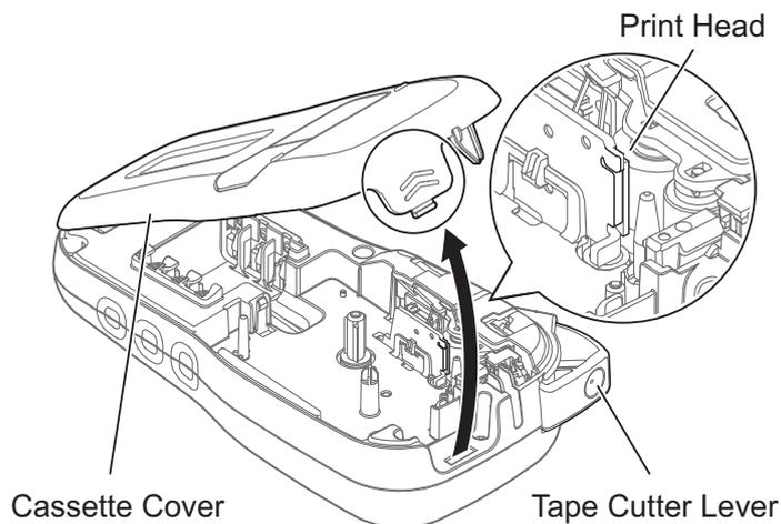
With the LCD facing down, open the Cassette Cover by pressing the grooved tab and pushing the cover in the direction of the arrow, as illustrated.
