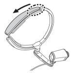
2 Slide the loop at one end of the rear band over the attachment post as shown in the illustration, and feed the rear band through the opening at the end of the head band.
