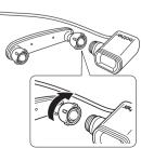
Turn the head band over so that the threads of the ball joint face the other way, and the AiRScouter logos on the head band covers are upside-down.
