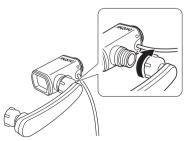
**8** Attach the flexible arm to the head band by lining up the wide end of the flexible arm with the threads on the head band, and rotating the dial on the ball joint clockwise to tighten.
