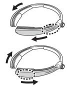
Attach the flexible arm for right-eyed viewing (the other arm that is included in the box) to the head display, by lining up the narrow end of the flexible arm with the threads on the head display and rotating the dial on the ball joint clockwise to tighten.
