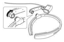
A Rotate the dial on the ball joint between the flexible arm and the head display clockwise, until the flexible arm is separated from the head display.
