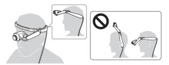
Note If the head band feels loose or starts to slip down the forehead, it is recommended that you attach the rear band and use it to tighten the fit on your head.
