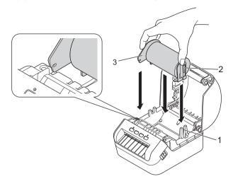
4 Thread the DK Roll through the printer.
