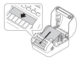
• Push the first label through the Label Output Slot until the end comes out of the Slot as shown.
