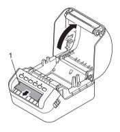
3 Place the DK Roll into the Roll Spool Guide (1).
