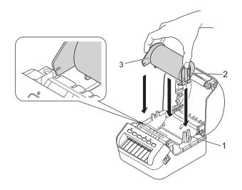
4 Thread the DK Roll through the printer.
