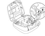
2. Install a new cutter unit. Push it in until it snaps into place.
